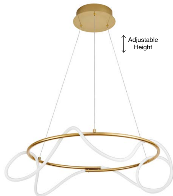
TIRIAC - 9548104 Triac Dimmable Gold Aluminium & Acrylic LED 43 Watt 230 Volt 4581Lm 3000K IP20 D: 70 H: 120 cm LED WARM WHITE DRIVER INCL.
